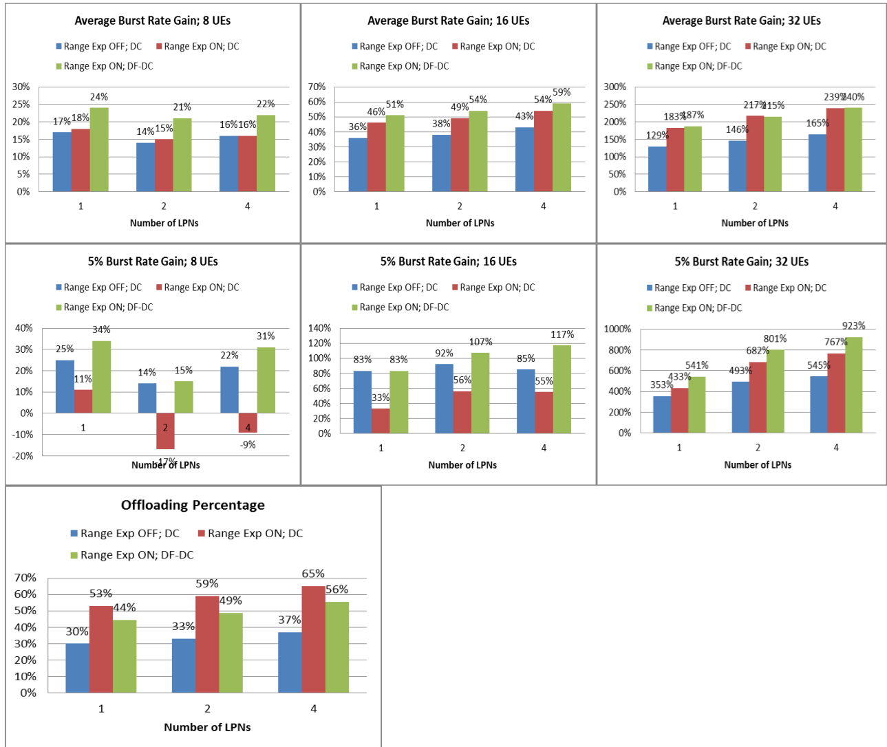
Figure 50: DL bursty traffic performance, 30dBm LPNs and 50% clustering dropping, 60% indoor UE
